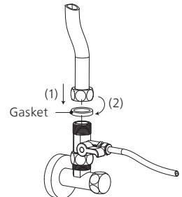
e. Switch off the three-way ball valve. Turn on the cold water supply. Wipe the connections with a tissue to see if there is leakage. If the tissue stays dry, it means the three-way ball valve is installed properly.
