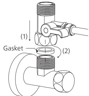
d. Connect the cold water hose with the three-way ball valve and screw it tightly with a wrench. Please don't miss the gasket in the cold water hose during installation.
